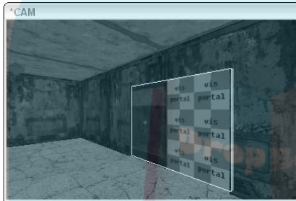
Figure 11-20: Placing a portal brush inside of a func_door creates a sealed area for better optimization.
